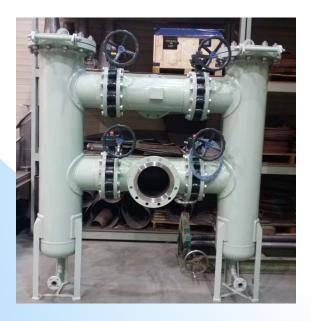
It is a duplex strainer with two independent filter screens connected.
