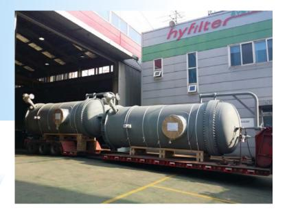
It is a container manufactured to withstand pressure for the purpose of storage, reaction, filtration, separation, etc. of liquid or gas.
