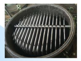
It is a device that filters the cake by individually mounting leafshaped filter elements in a vertical housing on the central manifold.
