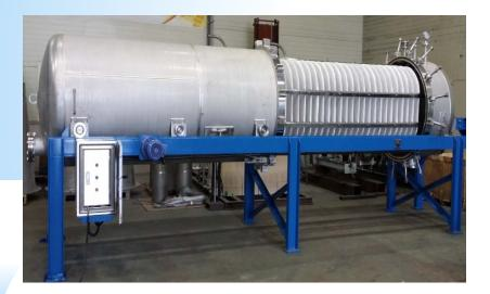
It is a device that filters a cake by individually mounting a leafshaped filter element in a horizontal housing on the central manifold and pressing the cake.
