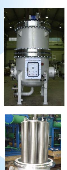
It is an automatic strainer that filters by installing a number of candle-shaped filter screens in a certain arrangement, and discharges impurities by differential pressure.
