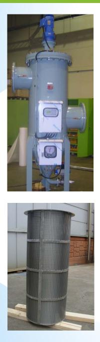
It is an automatic strainer that filters through a basket-shaped filter screen and discharges impurities by differential pressure.
