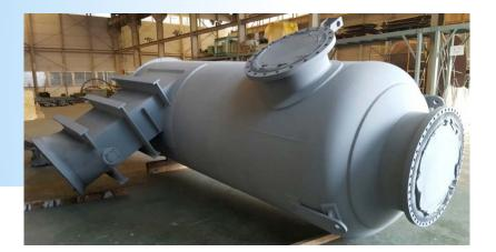
It is a device that removes liquid mist or impurities in gas or gas. It is equipped with a wire pad.
