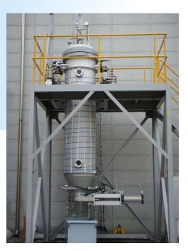
It is an automatic filtration device that filters and backwashes candle-type filter elements individually mounted on the manifold.
