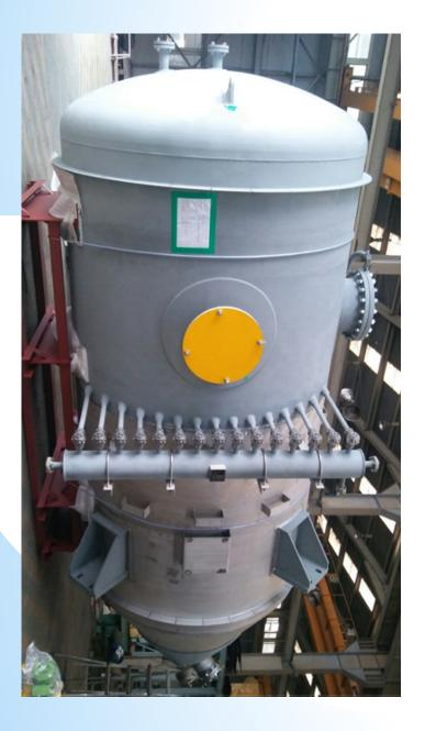
It is a dust collector that filters and discharges gas or gas containing dust.
